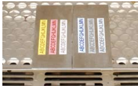
Temperature resistant: laminated labels were subjected to temperatures ranging from -80C to +150C for 240 hours, and the text was found to be unaffected
