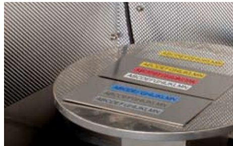
Fade resistant: after laminated labels were placed in a fade-inducing chamber to simulate a year in sunny surroundings, the text was unaffected
